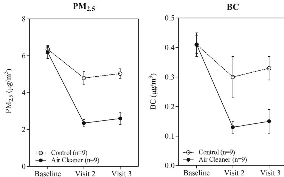
**FIGURE 2.** Classroom particulate pollutant levels. Classroom PM<sub>2.5</sub> ( $\mu\text{g}/\text{m}^3$ ) and BC ( $\mu\text{g}/\text{m}^3$ ) levels at baseline and follow-up visits in the intervention and control groups. Mean and standard errors shown.
